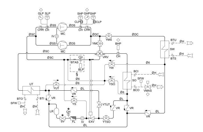
The SW6 unit, allows the production of cold and hot water, independently from the operation mode of the unit (heating or cooling).
