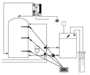
Correct positioning of the BTS sensor
