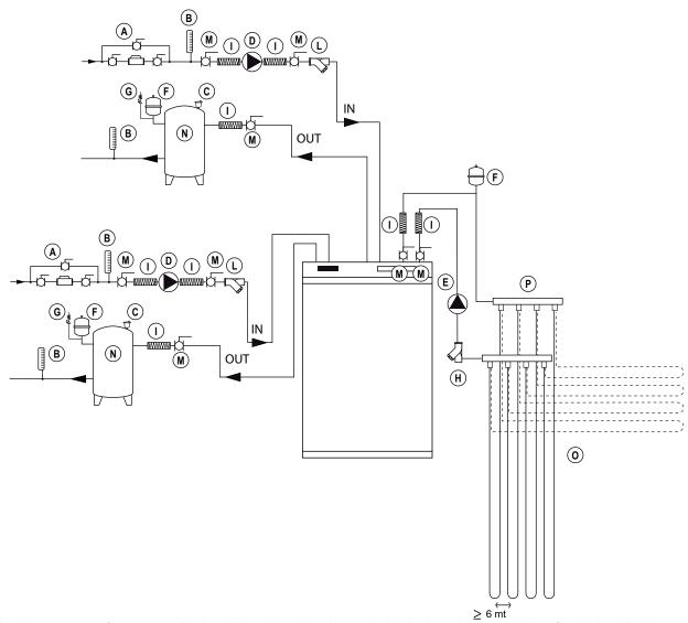
The above system refers to an application with geothermal probes vertical or horizontal. In the majority of vertical applications using PE pipes connected in parallel, placed at a distance of at least 6 meters. Normally the vertical perforations must be approved by local authorities. In case of horizontal applications will typically use PE pipes buried about 1.5 to 2 meters deep.
