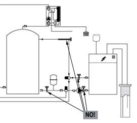
Incorrect positioning of the BTS sensor
