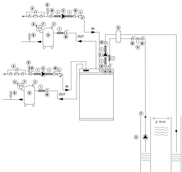
The system above is the most secure and reliable, involves the installation of an intermediate water –water plate heat exchanger which protects the source of the heat pump from clogging, corrosion and freezing.
