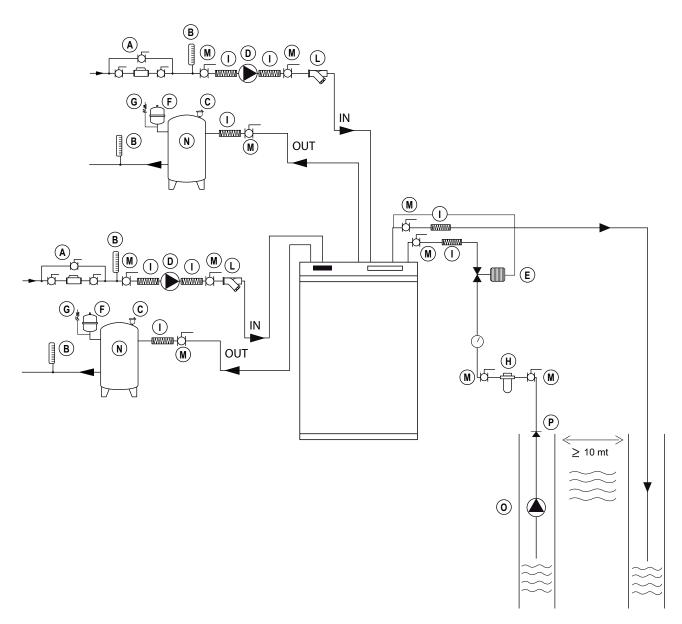
The above system is the most economical and efficient, but it can be used ONLY in cases where a water quality parameters are within the limits shown in the table. It is ALWAYS recommended to perform an accurate chemical analysis of water by a qualified technician. In the case where it is not possible to maintain control the water quality parameters listed above there has to opt for a source hydraulic circuit type 2.
